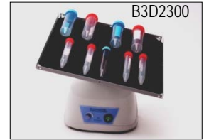
Variable Speed • Speed is adjustable from 2-30 rpm • Platform angle adjusts from 0-30° • Cold room & incubator safe (4-65°C) • Load capacity is 2 kg (4.5 lbs) • 2-year warranty; maintenance-free brushless motors 2-D (seesaw), 14 x 12" platform w/flat mat BenchRocker™ 2D. BR2000 ..... $712.00 3-D (nutating), 12 x 12" platform w/dimpled and flat mats BenchRocker™ 3D. B3D2300 ..... $663.00
